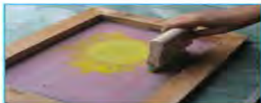
CdS paste deposition on Si substrate by screen printing method
